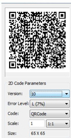
**QR Code Parameters:** You can set QR Code image parameters before being inserted.
