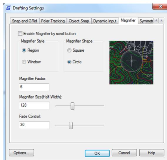
Enable Magnifier by Scroll button: If you check this option you can enable/disable the magnifier command by clicking the scroll wheel of the mouse. Also the shortcut key Ctrl + E is available to activate magnifier.
