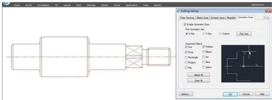
It is possible to directly draw symmetrical shapes with Symmetric Draw tool. When drawing the first half you get another half automatically. The default symmetry axis is X-axis, but user can specify Y-axis or any line in the drawing as symmetry axis reference.
