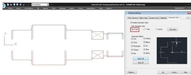
**Y Axis option:** The objects drawn will take the Y coordinate system as invisible axis line. The effect of Y Axis is mirroring the drawn objects right or left side according to Y coordinate system origin location.
