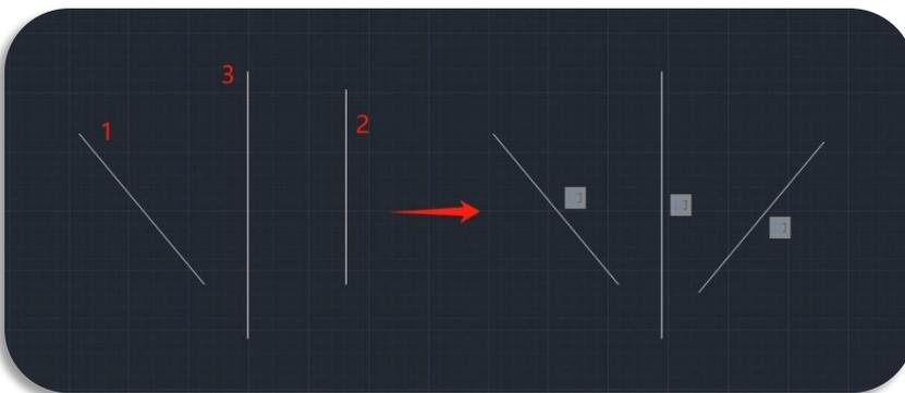
(12) **Equal**: Constrains two lines or polyline segments to maintain equal lengths, or arcs and circles to maintain equal radius values
