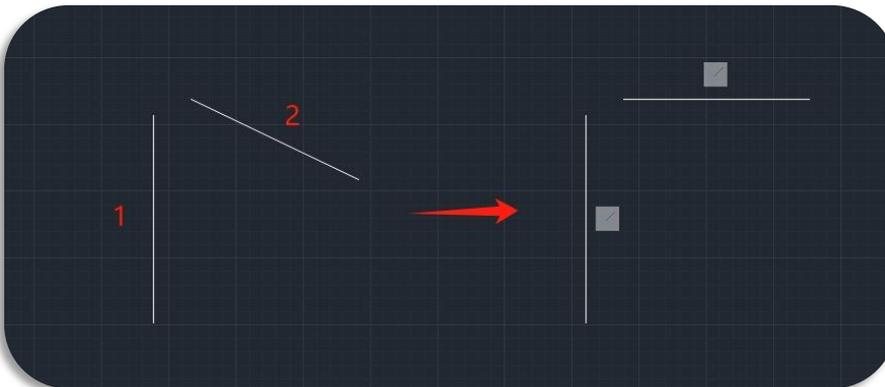
(7) **Horizontal:** Constrains a line or pairs of points to lie parallel to the X-axis of the current UCS.
