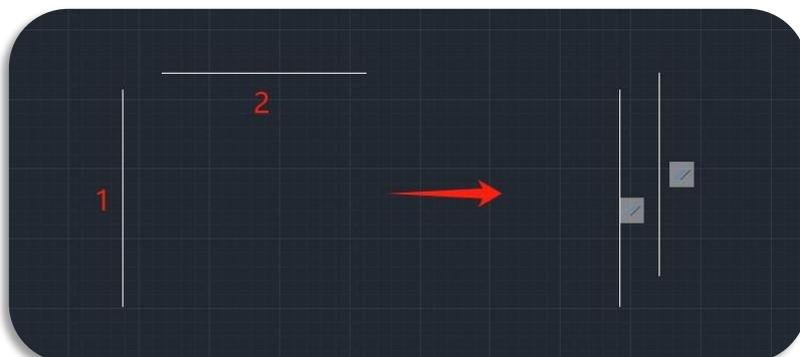
(6) **Perpendicular:** Constrains two lines, or polyline segments to maintain a 90-degree angle to each other
