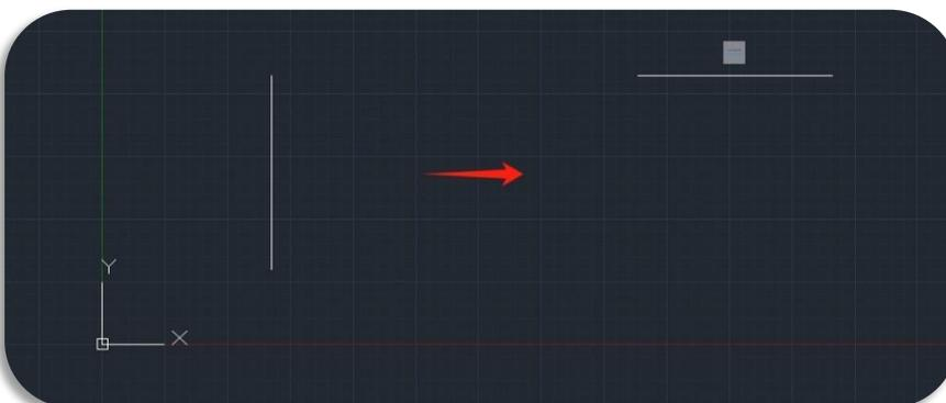
(8) **Vertical:** Constrains lines or pairs of the points to lie parallel to the Y-axis of the current UCS.
