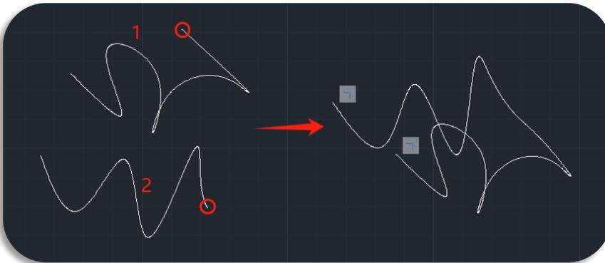
(11) **Symmetric:** Constrains two curves or points on objects to maintain symmetry about a selected line.
