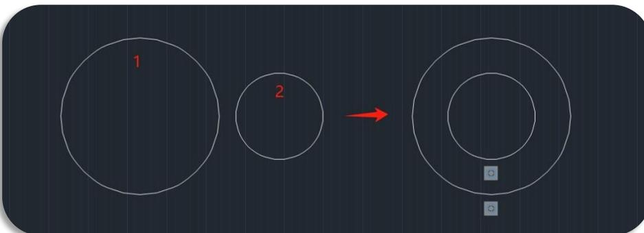
(4) **Fix:** Constrains a point or a curve to a fixed location and orientation relative to the World Coordinate System.
