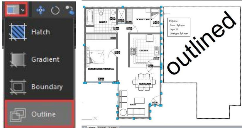
For example, use this tool extract the outline shape of a floor plant house to later calculate its total area or to reference draw the roof of it.
