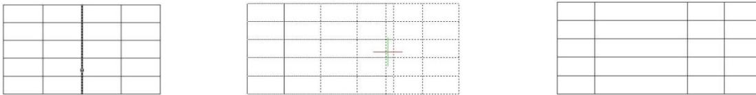
**Drag Line:** Different to Multiline drag, Drag line will just move the line you selected and other relevant lines will not move.
