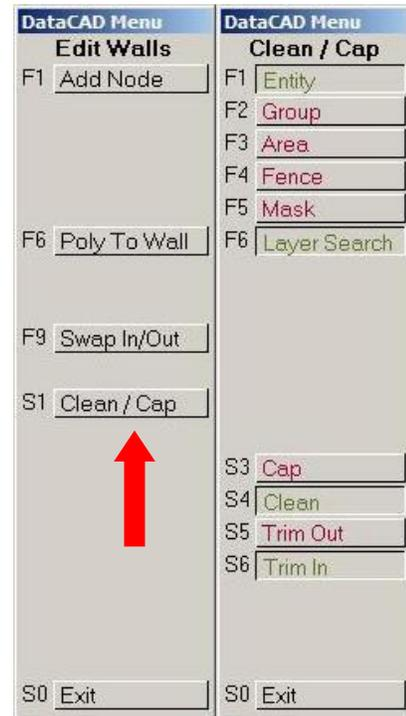
When you select walls to change by Entity, Group, Selection Set or Select All both nodes are changed for each selected wall. If you select by Area or Fence, only the wall nodes that are enclosed within the selection rectangle or polygon will be selected.
