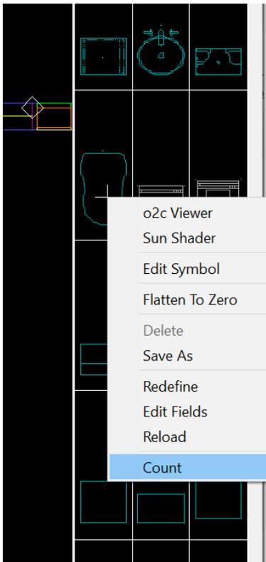
In the case of Smart Doors and Windows, instances of non-fixed width types of varying widths are tallied separately. So, the count will only include instances of the current type with the current width.
