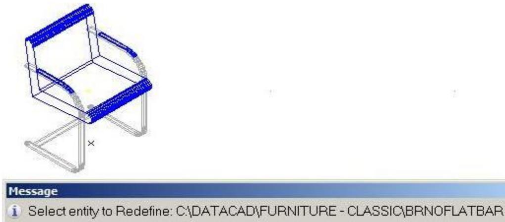
DataCAD has a new "Auto Reload" option, located in the [Ctrl]+[Right-click]/Symbol Tools context menu for symbols. When this option is checked, DataCAD will automatically reload the symbol definition on the hard drive for each instance of the selected symbol every time you open the drawing. This setting is assigned and remembered on a per-symbol (but not per-instance) basis.
