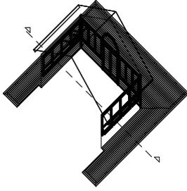
The cut line is a series of dashes; the arrow indicates the view direction
