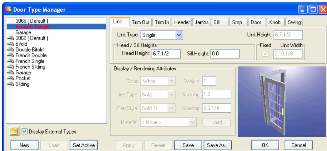
3. Refine the door properties by using the options in the various tab sections of the Door Type Manager.
