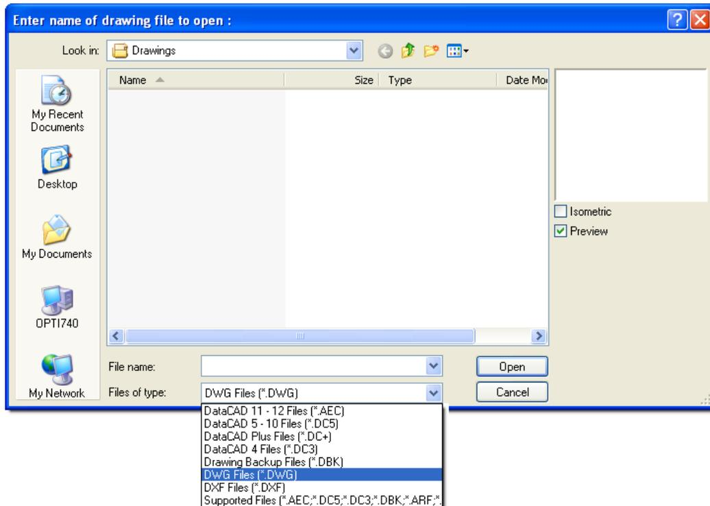
3. Select a file to import from the list or type the name of the file to import in the File name input box. By default, DataCAD looks for DXF and DWG files in your DataCAD\Transfer folder. If your DXF or DWG files are in a different folder, change to that folder using the “Look in:” drop-down and then click on the file you want to import.
