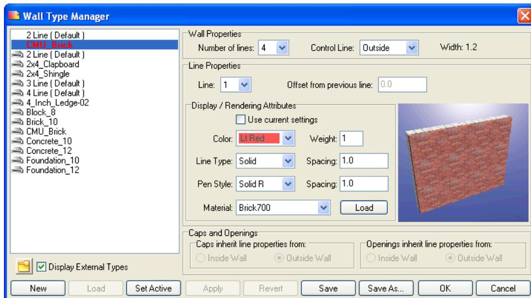
5. Select the wall type you would like to use instead of the default by double-clicking or by highlighting it and clicking on Load. Notice that when you make a selection, the illustration in the preview window and the wall and line properties change.
