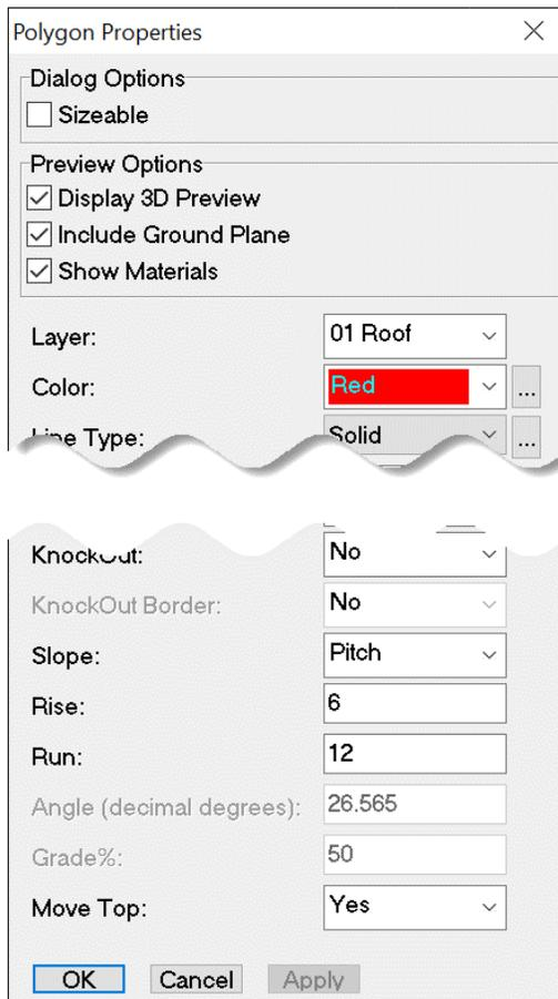
The Entity Properties Editor has been updated to include the Slope parameters of 3D Inclined Polygons and Slabs. When you display the properties of a 3D Polygon or Slab that is not horizontal or vertical and has at least one edge parallel to the ground plane, its slope properties are shown.
