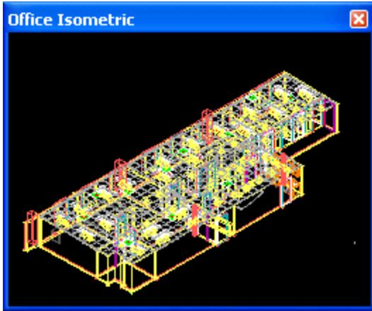
To turn Multi-View Windows on, open your drawing and choose "Toolbars" from the "View" pull-down menu. Place a check mark next to each window that you would like to display. Alternatively, you may open the drawing and press [Ctrl]+[w] on the keyboard to turn on all Multi-View Windows.
