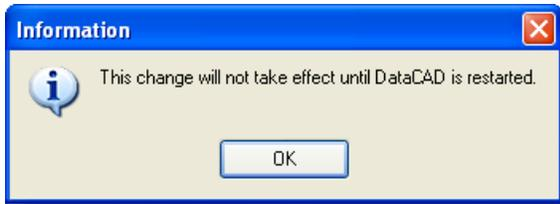
To enable this feature, open the Layer Manager in a drawing and click the check box which says, "Keep Layer Manager Open." You will need to exit and reopen DataCAD for this setting to take effect.
