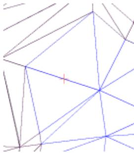
5. Click on the line that separates two adjoining triangles. DataCAD flips the valley.
